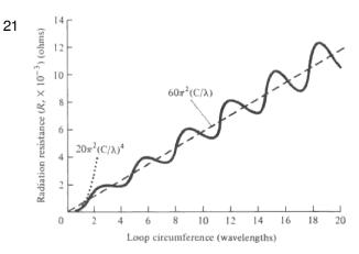
The radiation resistance of the loop antenna is rather low. Without changing the size of the antenna or wavelength, how can the radiation resistance be increased?
